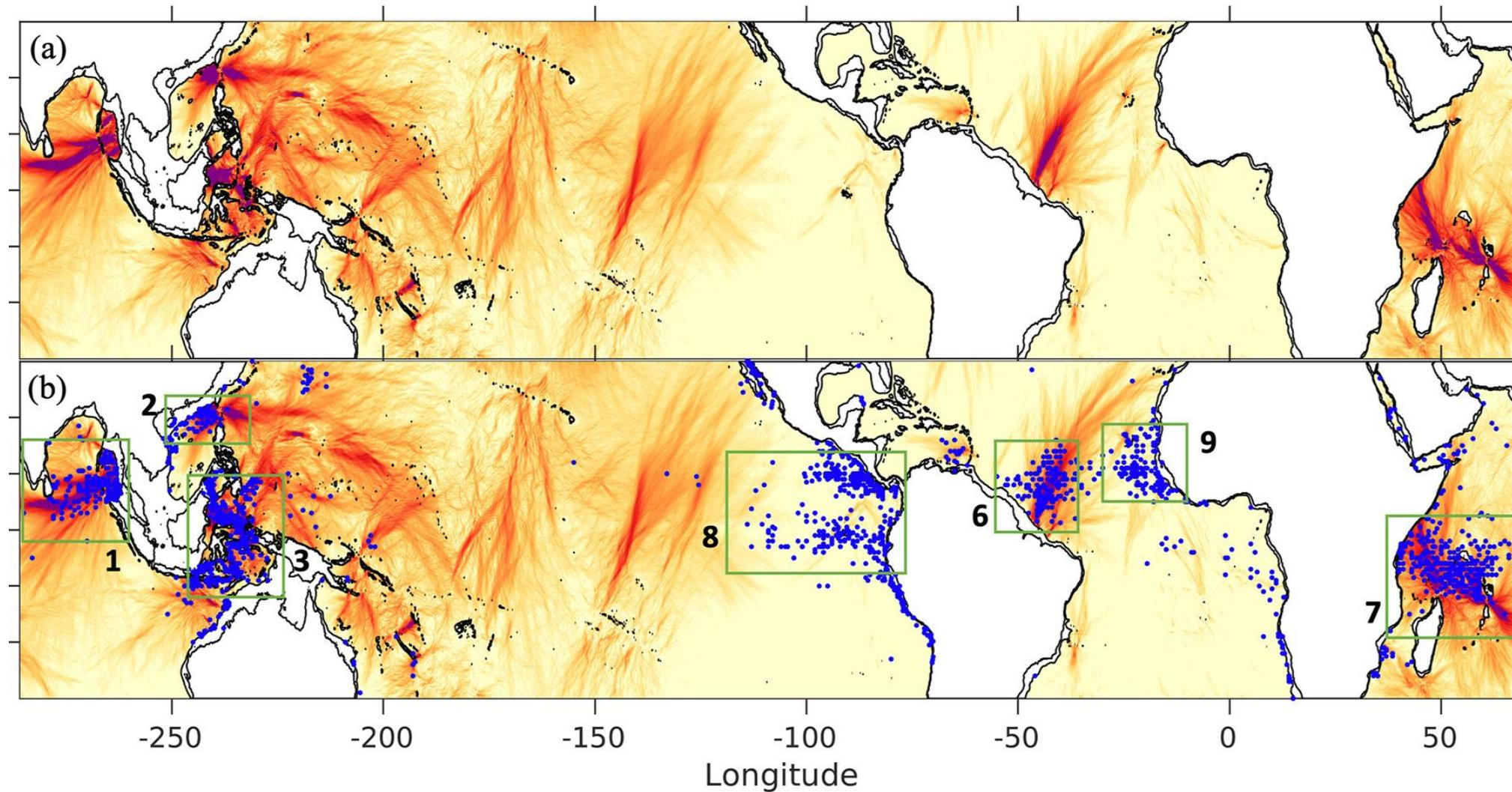
(a, b) Colormaps of time-mean and depth-integrated supertidal energy fluxes in global Hybrid Coordinate Ocean Model on a logarithmic scale compared with (b) observations of nonlinear internal waves (blue dots) captured by 250-m resolution Moderate-Resolution Imaging Spectrometer imagery. [Solano et al., 2023](#).
