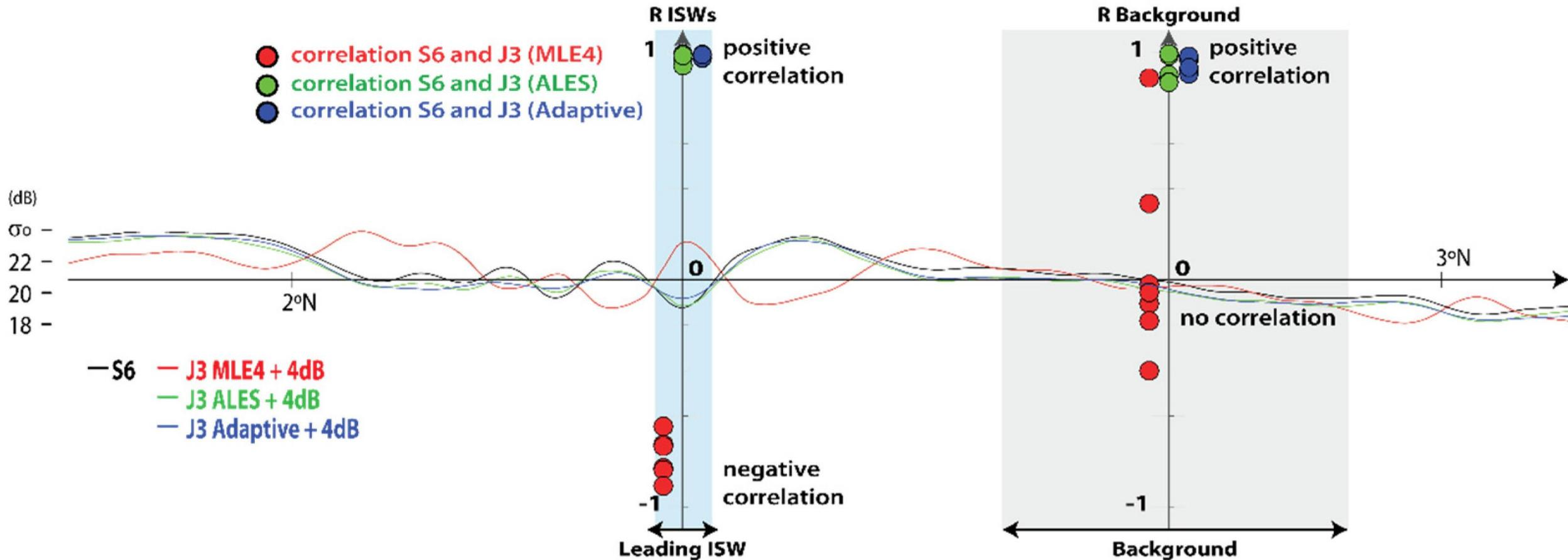
Green and blue circles represent correlations between Sentinel-6 and Jason-3 (ALES/Adaptive, respectively), and red circle represent correlations between Sentinel-6 and Jason-3 (MLE4). Two sets of correlation coefficients are shown, listed as follows: on the left for the leading ISWs ( $R_{ISWs}$ ), and on the right for the waves' background conditions ( $R_{Background}$ ). A representative case is shown for the Celebes Sea using data smoothed with a running mean of about 10 km.
