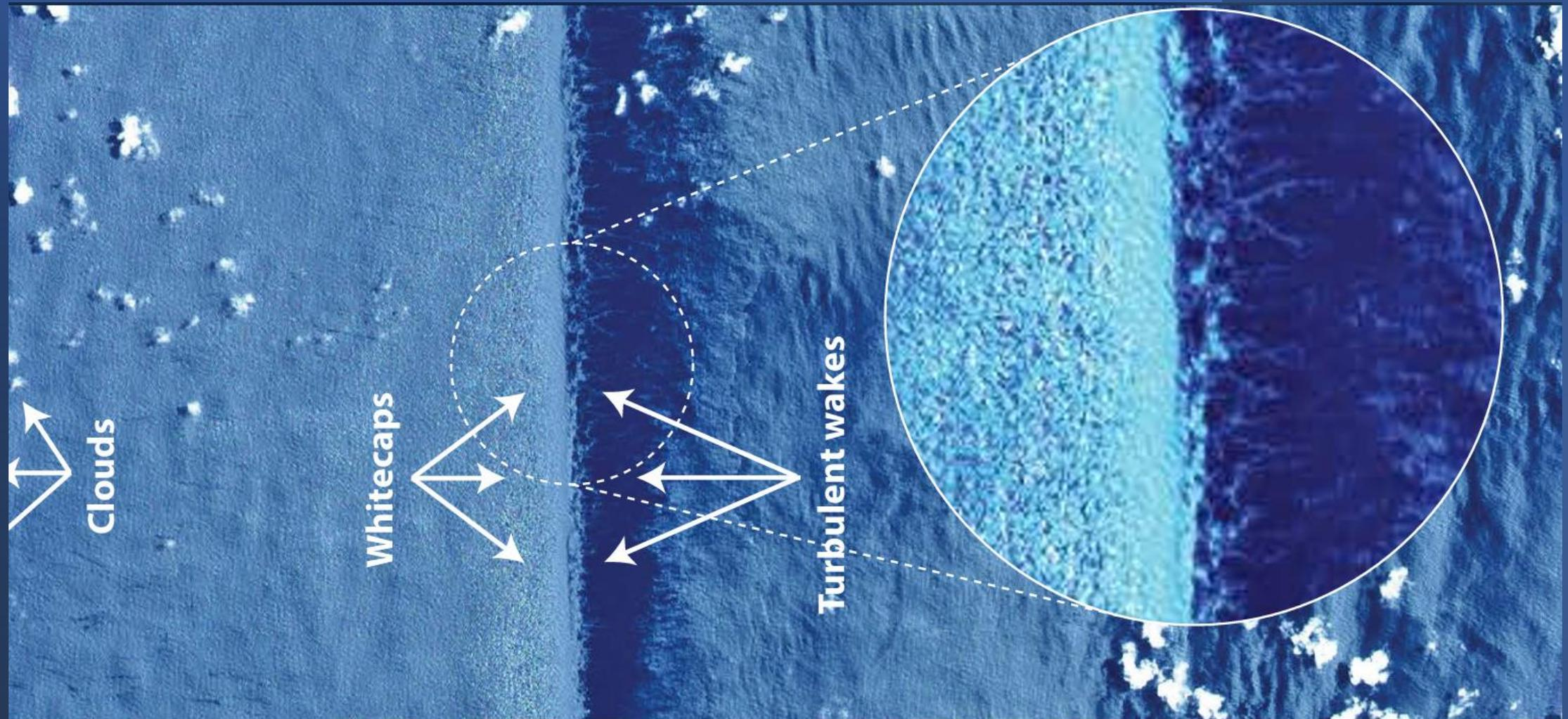
Sentinel-2 optical image (<https://odl.bzh/sPxDcyYH>) highlighting the surface turbulence of a large-scale internal solitary wave propagating in the South China Sea (from right to left). Note the whitecaps ahead of the wave and the smooth (slick-like) section behind it (in dark blue), and what appear to be the turbulent wakes (visible as whitish filaments of foam) that stretch from the whitecaps into the slick-like section.
