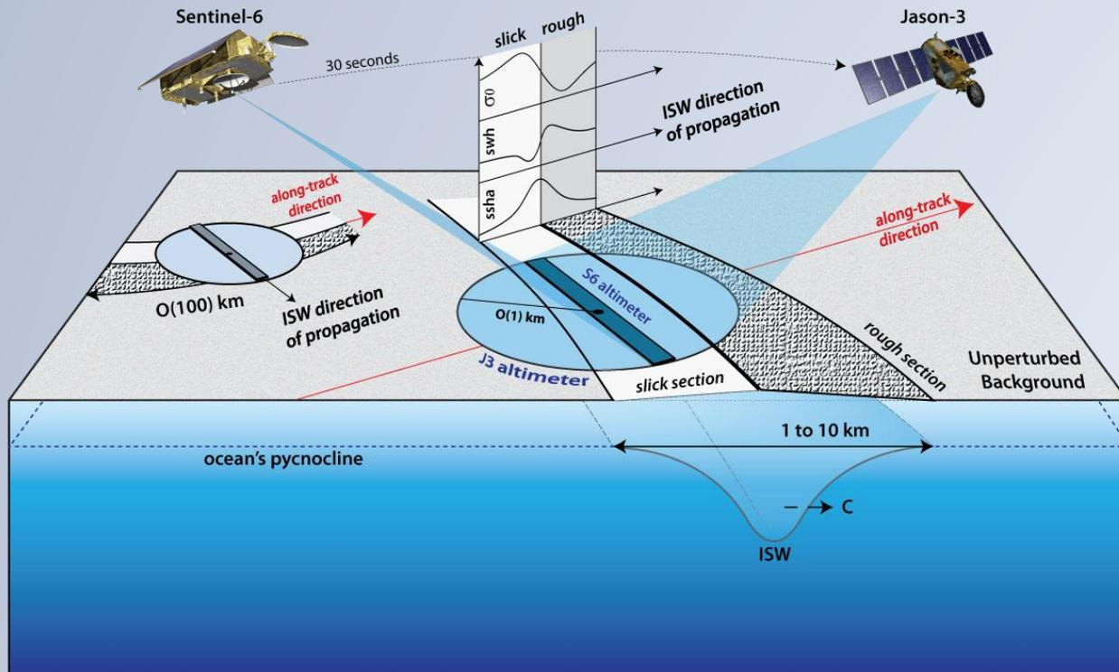
It's just a matter of sampling. The larger footprints in the conventional altimeters get mixed contributions in scales between 1 and 10 km, while SAR altimeters seem to be able to sample them correctly. However, both seem to fail close to scales of about 1 km or if there is a bad alignment between features and altimeter.
