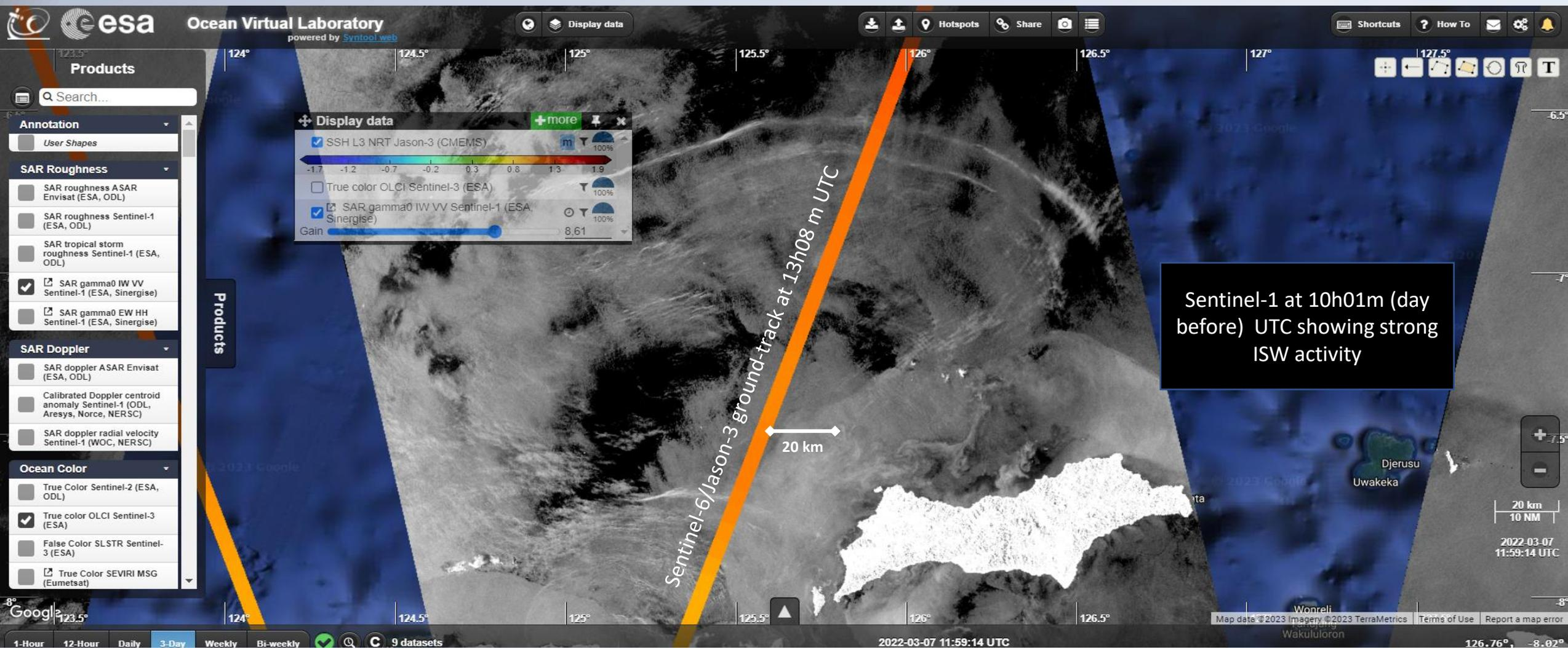
In the Banda Sea we know that we have ISWs that are larger, farther apart, and conveniently aligned with the altimeter ground track
