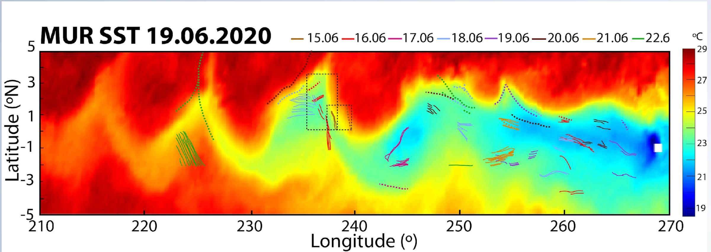
Spatial distribution of the fronts (dotted lines) and ISW packets (solid lines), identified in the visible imagery of Sentinel-3, between 15 June and 22 June 2020. The colour for each day is identified in the upper part of the map. The dashed dark rectangles show the location of some OLCI images given in Santos-Ferreira et al. (2023). A MUR SST image, dated 19 June 2020, is shown in the background.
