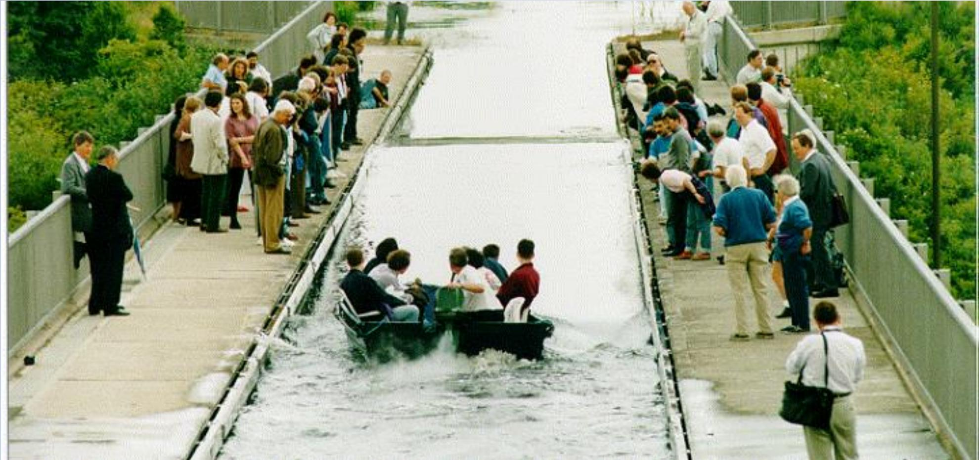
A surface soliton is shown propagating in a narrow water channel, which was recreated in an experiment similar to that of Sir Scott Russell in 1834. Note how the solitary wave propagates ahead of the boat as it decelerates and comes to a full stop. See more at <http://ramanujan25449.blogspot.com/2017/05/solitones.html>.
