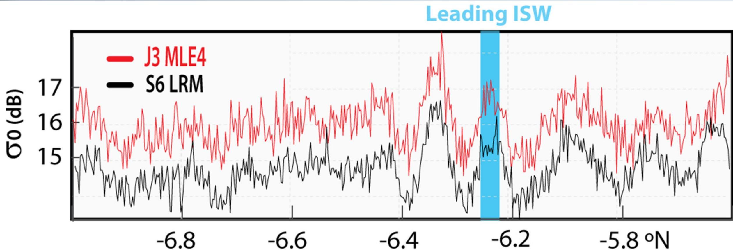
Comparing  $\sigma_0$  for Sentinel-6 (S6) level-2 products (at 20 Hz) in LRM (i.e., conventional altimeter) modes, and data from MLE4 in Jason-3 (J3).
