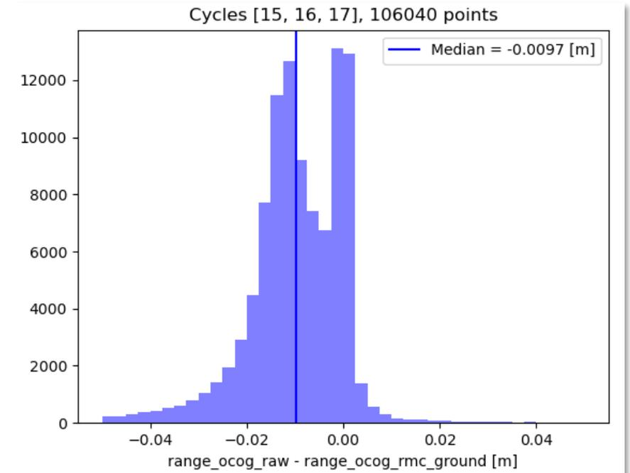
*Distribution of the differences in between the range derived from the RAW and RMC waveforms with OCOg retracker*
