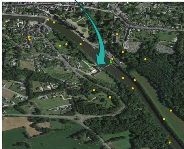
Green = in situ station position, yellow = position of the nadir of successive cycles altimetry data
